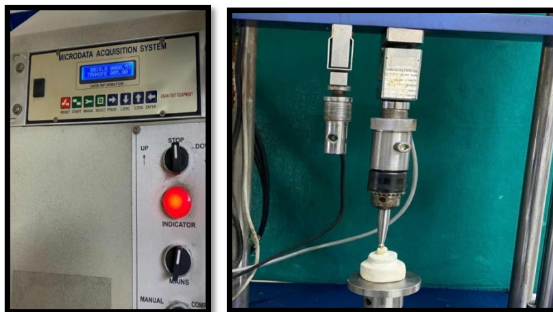
Figure 2: Axial loading of 10 Kgs during cementation with the help of universal testing machine
