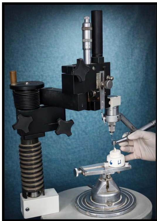
Figure 1: Tooth preparation with the help of surveyor and attached custom made metal Jig
