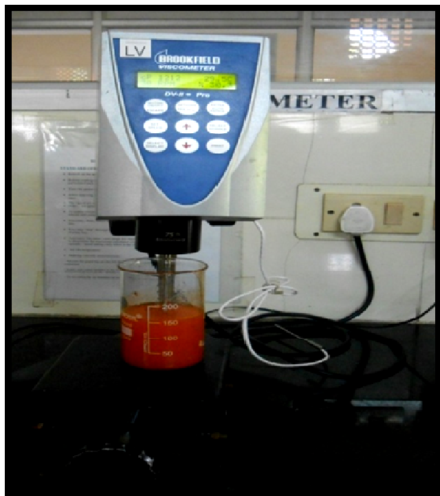
Figure No. 1: Brookfield viscometer displaying viscosity value
